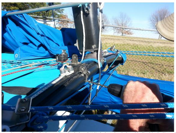
Another view of swivel cam cleat for halyard (10), below that halyard bullet block (9), to the right of that crossbar/pole attachment (1), and to the right and below that (barely visible) plastic eye strap (11)
