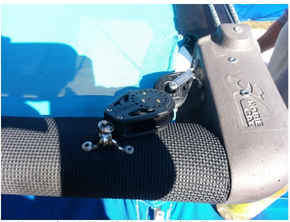
{Looking center from STARBOARD side at FRONT of siderail} Ratcheting sheet block (6) on siderail and sheet cheater block (7) on FRONT casting
