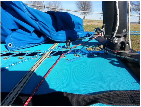
{Looking center from STARBOARD side} Near center of pic is halyard retriever pulley/plate (5) and to the right swivel cam cleat for halyard (10)
