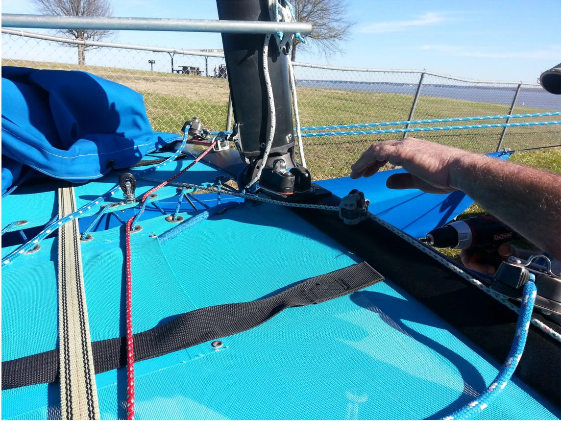
Another view of halyard retriever pulley/plate (5) and swivel cam cleat for halyard (10)
