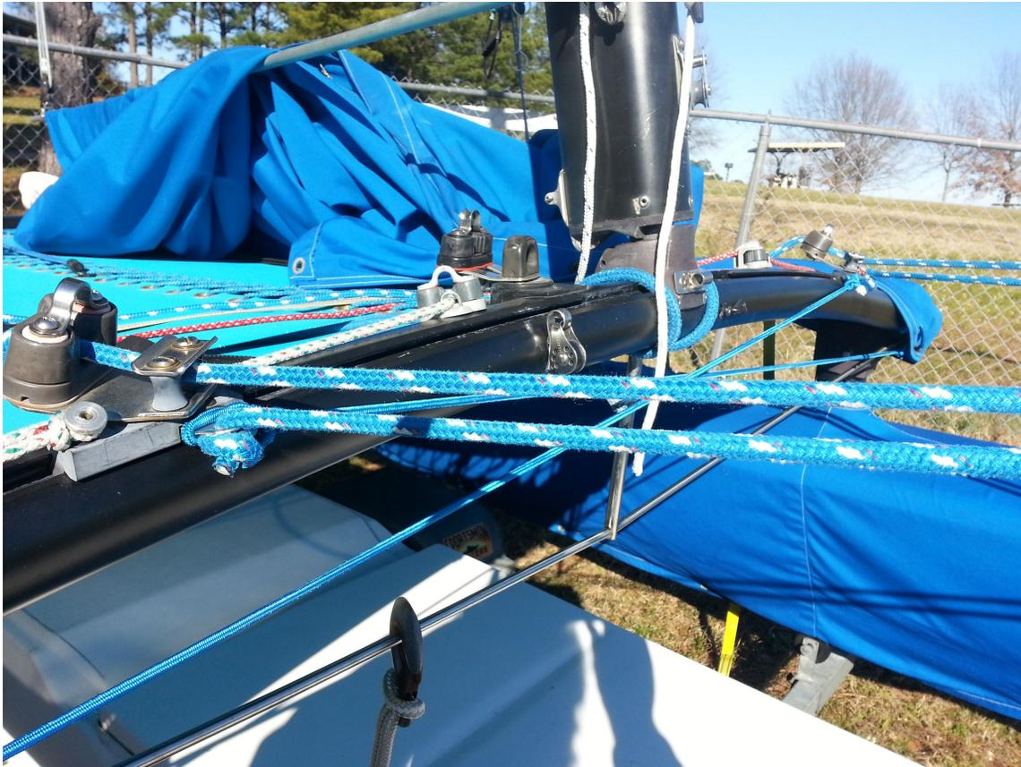
{Looking AFT from STARBOARD, FRONT side} Near center of pic is swivel cam cleat for halyard (10), below that halyard bullet block (9), to the right of that crossbar/pole attachment (1), and to the right and below that (black, hard to see) plastic eye strap (11)
