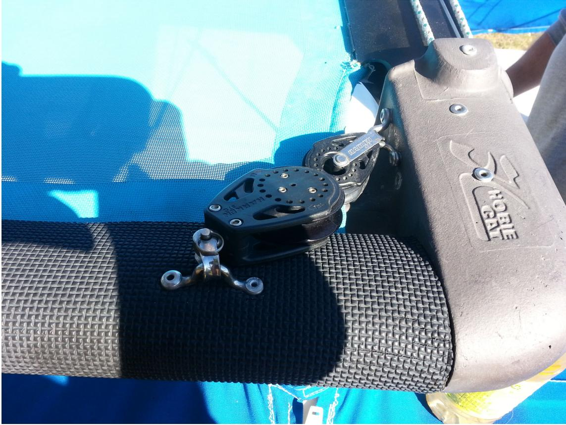
{Looking center from STARBOARD side at FRONT of siderail} Ratcheting sheet block (6) on siderail and sheet cheater block (7) on FRONT casting
