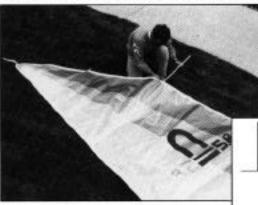
Slide the battens into the pockets making sure the batten tips fit snugly into the plastic caps riveted to the sail luff.
