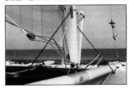
61. Using the extra 7 piece of shock cord supplied, attach the center to the mast and tie each end to dolphin striker bar on opposite sides of mast. Be sure the jib sheet is lead outside shock cord. This will keep the jib sheet from catching under mast base.
