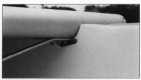
eted to the inside of the hull just under the forward chock). Rotate the main beam so that the beam hole will align with the 5/16" hole tapped in the main beam chock. Note: Do not install internal beam casting yet.
