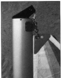
38. Mount jib halyard to mast using the wire block supplied with halyard. Be sure that halyard is oriented properly, with shackle away from mast, to travel down forestay. The jib halyard tail is 21" and ties to the free end of the jib halyard. Position both halyards on the mast with the shackles near base and tie off temporarily.
