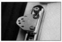
27. The parts are included in a separate bag. The jib cars have installed pad eyes. Remove the pad eye as it is not necessary with this system. Remove and mount jib adjuster plate to both hulls.
