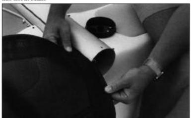
5. Gradually and equally slide both sides of the trampoline into the rails on each hull. Pull both sides of the trampoline aft so that the trampoline is fully engaged in the rails and the main beam rests loosely in the chocks. Insert PVC tube in slot at rear of tramp.
