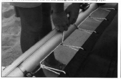
Take second lace line and begin lacing side tramp grommets from the main beam aft.
