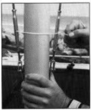
WARNING: If the diamond wires are too loose the mast could break under high pressure loads. Be sure to tape the locking nuts on turnbuckles after you have adjusted the wires so that they will not loosen.
