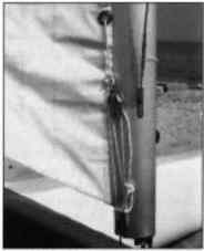
Attach the '/-' x 6' Downhaul lines to strap eye on mast. Feed through lower sheave on V-jam block, back down around block on mast up through V-Jam top sheave and tie knot in end to prevent it from undoing itself accidentally.
