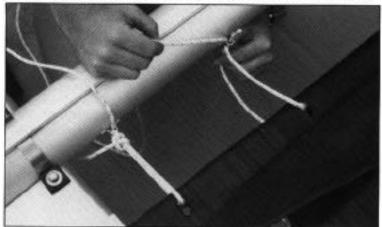
Repeat this procedure until the trampoline is laced. Go back to the beginning and pull the line tight as possible so the trampoline pulls taut at each eye in succession. Tie off the lacing line at the last strap eye.
