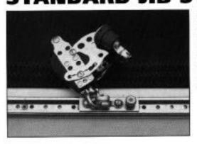
Attach jib block to pad eye on side jib tracks, or wire on 4-way system.
