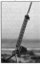
Assemble by pushing clevis pin forward through tack hanger, stay adjuster and forks. Secure with split ring.
