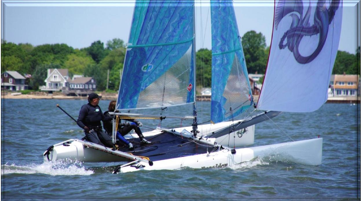
PE05 3.0 mil Injection prototype main and jib. Formulon F75 spinnaker with SailPrint.eu printed artwork.
