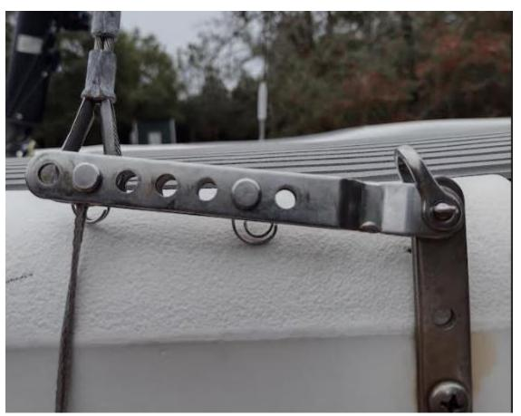
In this picture, the shorter shroud (thimble) is in its optimal loose rig position. The other pin is located at the optimal position for the longer shrouds. Again, these are not 'set in stone' settings but simply a guide for your starting point. Instead of twisting your hand on the wire, this is a better way to view the tension. This method makes it really easy to check other rigs when walking through the boat park and your curiosity is peaking!
