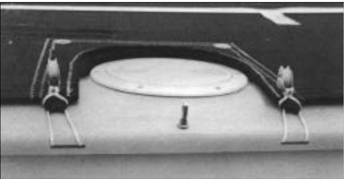
Slip tails of line under tab to hide and keep knot from loosening. Blocks should stand straight up.
