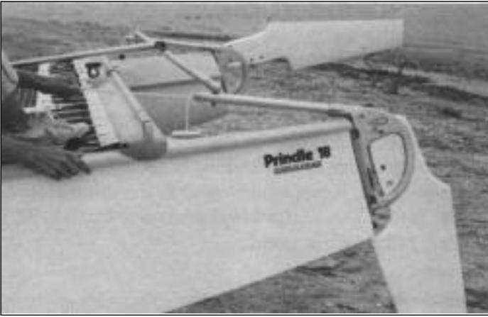
To lower rudder, release uphaul line from jam cleat and pull ball at end of downhaul line until lock bolt engages spring loaded pin in rudder casting.
