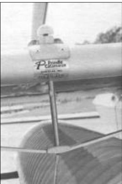
Loosen battens when storing the sail for more than a few weeks or during extreme temperature changes. This relieves pressure on the sail and battens and will preserve the life of both.
