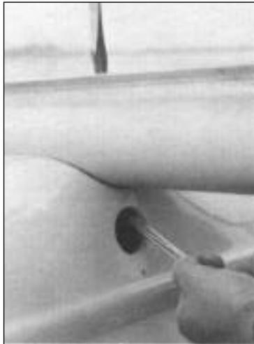
To attach outside bolts on both crossbars, insert 5/16" hex head bolt with washer through crossbar and deck. Insert through 6" stainless steel bar which fits under the deck. Hand tighten. Repeat procedure on all outside bolts.
