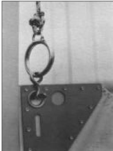
Attach the twisted shackle to the head of the mainsail and place forward edge of sail into curf of mast.
