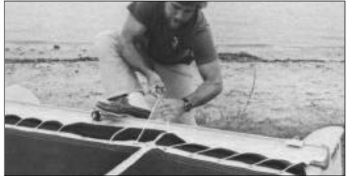
Stand at the back of the boat and tighten lines by bracing your foot against the rear crossbar for leverage. Pull as tight as possible. Tie off lines under trampoline. Do not trim excess line as this leaves something to hold when retightening tramp.
