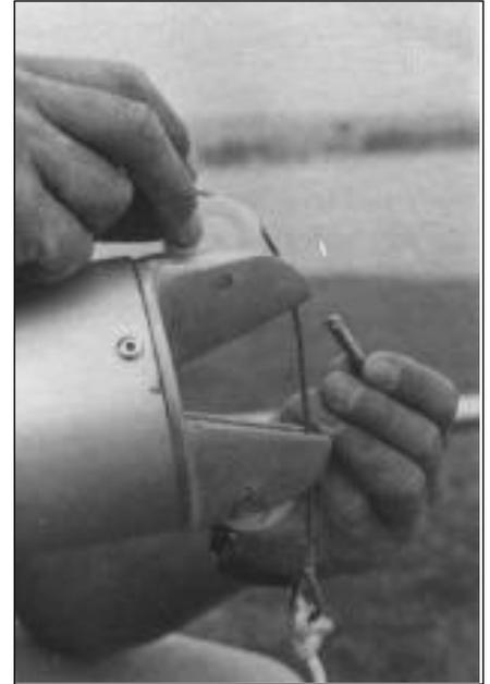
Attach main halyard line tail to eye of main halyard wire with bowline. Tie off main halyard line and wire to the base of the mast.
