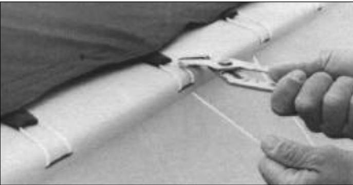
Tighten each side by using a pair of pliers or vice grips. Start tightening from the front and move to the rear. Be sure to get trampoline centered on boat by lining up the grommet nearest the front crossbar with the center of the mast step. Trim and burn excess line. Save for use later.
