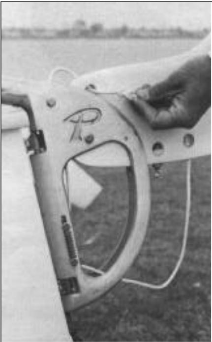
Insert 1/4" bolt through casting and 1/4" hole in rudder blade. Replace locknut and tighten until rudder will just fall by itself. Do not overtighten as this will restrict rudder movement, to loose and rudder will be sloppy in casting. Thread downhaul and uphaul lines into rudder blade and tie off ends with a figure eight knot. Make sure the ends do not extend beyond the edge of the blade. Follow same procedure on both blades.
