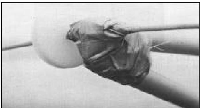
**DANGER! SPECIAL ATTENTION:** *Be sure all spreader fittings are securely attached. The mast will break if the diamond wires come loose. The mast is not covered under warranty for breakage due to improper tuning, assembly or maintenance.*
