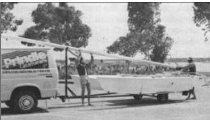
While the second person holds the mast, remove the hinge pin and walk the mast forward until you can place it in the front mast
