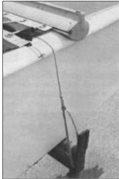
Place the boat on the trailer. Tie the boat down using at least 1/4" nylon or dacron line. DO NOT TIE ANYTHING TO THE DOLPHIN STRIKER OR ROD. Remove the rudder blades from castings. Be sure they are marked port or starboard so you don't have to retune them the next time you go sailing.
