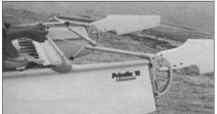
To raise the rudder, grab handle at end of tiller and pull until desired height of rudder is achieved.
