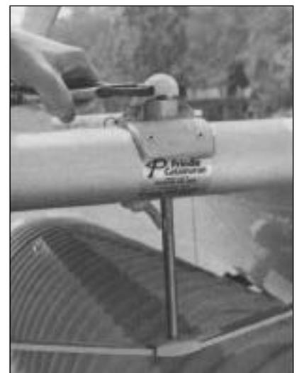
Loosen screw at bottom of striker rod.
