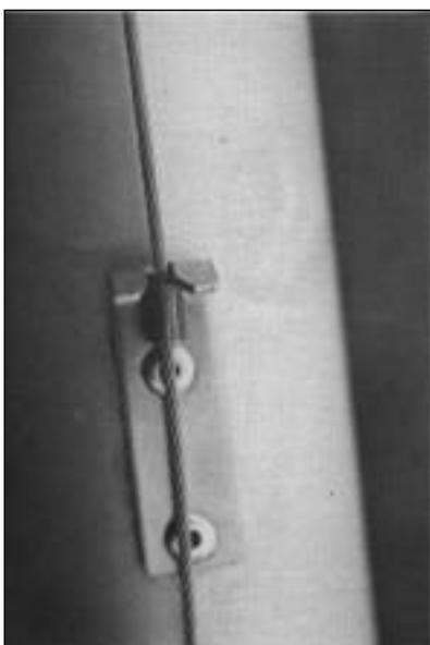
When the sail reaches the top of mast, you must secure the second metal stop on the halyard wire into the halyard lock on the mast. DO this by leading wire between teeth on lock and pulling down on sail to put tension on the metal stop. The other stop, further down on the halyard wire,
