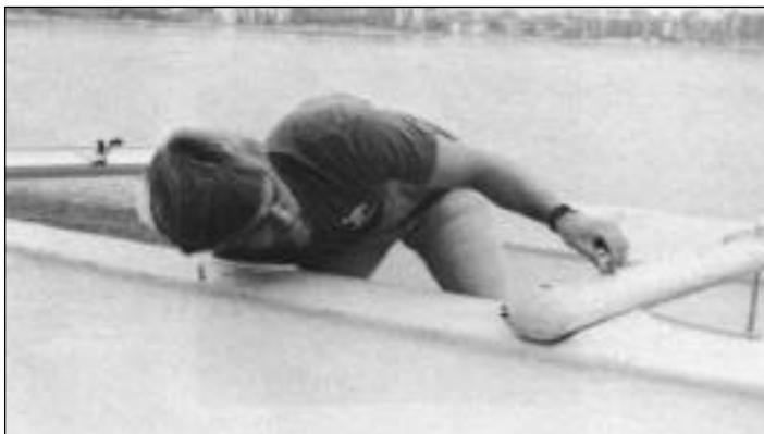
To attach inside bolts on the front crossbar, insert 5/16" hex head bolt with washer into inboard hole in crossbar and through the bolt
