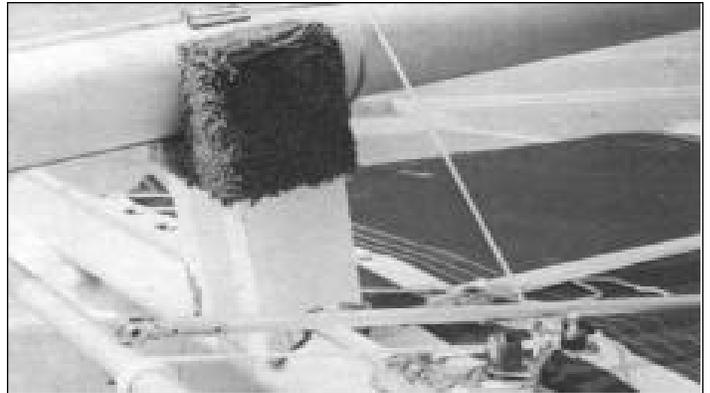
Secure the mast and support to the boat by wrapping the tie down line around the mast twice and down through the trampoline grommets. Store the tiller under a hiking strap or jib lead line to keep it from flapping around. Tie a 3 or 4 foot piece of line to the traveler pad eye, around the tiller crossbar twice, and through the fairlead and cleat. This will keep the rudder castings from swinging. Tie the front end of the mast down making sure to wrap line twice here also.
