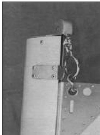
When the sail reaches the top of the mast, you must lock the ring on the halyard line to the hook at the head of the mast. To do this, pull halyard until the ring is above the hook.
