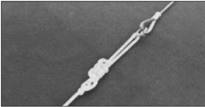
Attach jib blocks to thimble at end of jib bridle wire (not shackle) using 3/16" shackle. Be sure the jaws of cleat face inboard. Thread 5/16" x 33' jib sheet line by tying off one end to jib block with bowline. Thread through small jib clew blocks, through cleat on jib block, across tramp and through opposite jib block in opposite direction. Jib sheet should be one continuous line.
