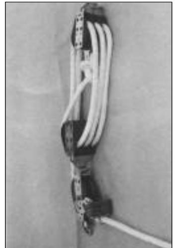
All boats: Install upper block to block hanger on boom with 1/4" shackle. Install lower block to traveler with 1/4" shackle.
