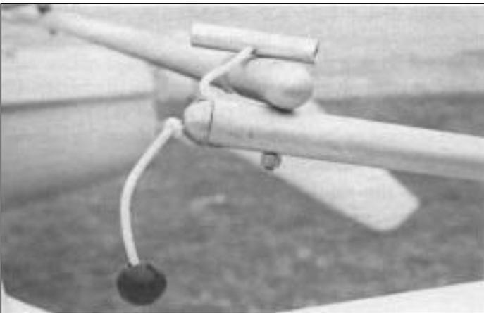
In operation if the rudder is pulled up too far, the head of the rudder blade will hit the washers at the top of the casting. This could chip your rudder blade. To prevent this, tie a knot in pull down line about 3" from ball. Adjust position of knot so that the raised rudder stops just short of hitting the washers.
