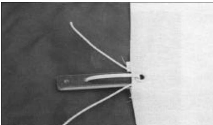
Lead string up through either hole in foam batten or through end cap and down through top grommet and tie an overhand knot (tightly) while pushing batten into sail with thumb.
