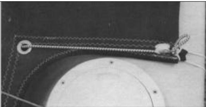
Lead shock cord through block, down through grommet by hatch and up through grommet and block on opposite side of tramp. Secure end until needed later.
