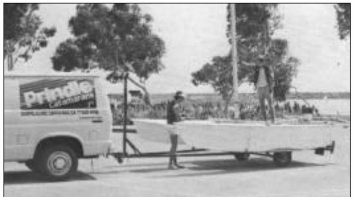
Attach mast hinge to the mast. With one person on the trampoline, push the mast forward and disconnect the forestay shackle. DO NOT undo the turnbuckle. Rig shackle so it holds the two bow bridle wires together. Check in back of boat to make sure you will not be lowering the mast onto a person, car, or power line.
