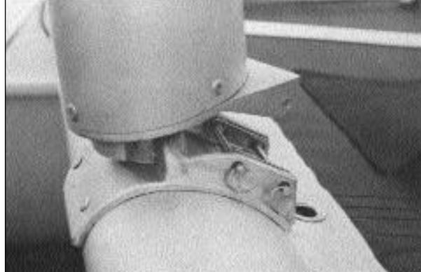
Prindle 16 mast step hinge in use
