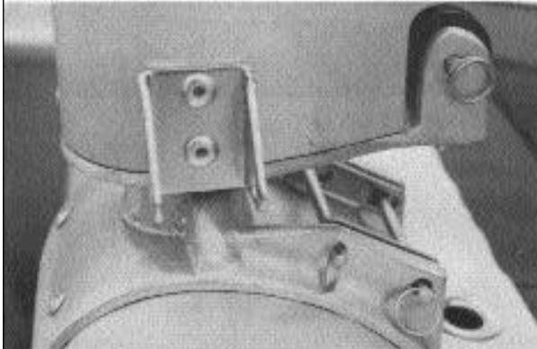
Prindle 15 mast step hinge in use
