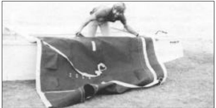
From the port hull, insert forward and rear edges of trampoline in curfs on crossbars. The rear edge has two rows of grommets.
