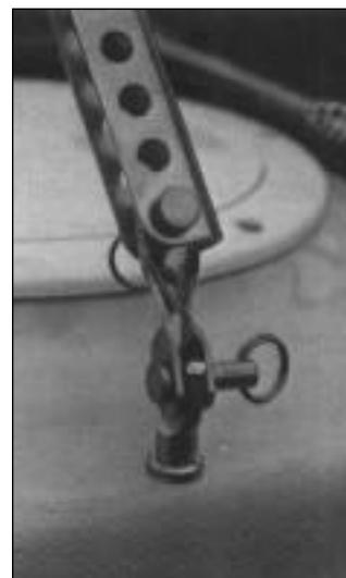
Tie a trapeze ring to each of the 3' lines supplied. Thread the line through the thimble at the end of the trapeze wire. Thread one of the plastic height adjusters onto the line, wrapping the line around it at least twice. The adjuster allows you to adjust your trapeze height. Tie the tail of the line to the shock cord with a bowline.
