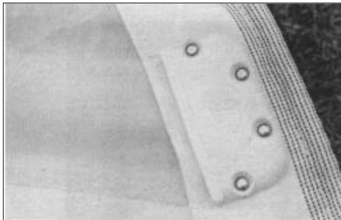
Insert tapered end of each batten (foam core) or the end with rounded edges (fiberglass) into batten pockets making sure each batten fits into the pocket end protector at forward edge of sail. Put plastic caps on aft end of fiberglass battens.
