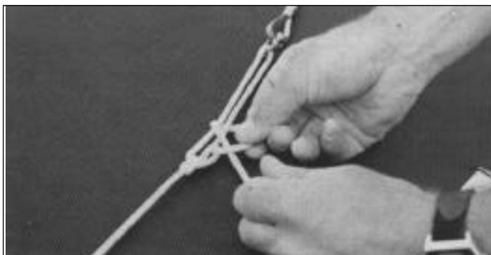
Using a truckers hitch, tie the line to the 3/16" shackle on opposite jib bridle wire. Pull line as tight as possible and tie off using a row of half hitches.
