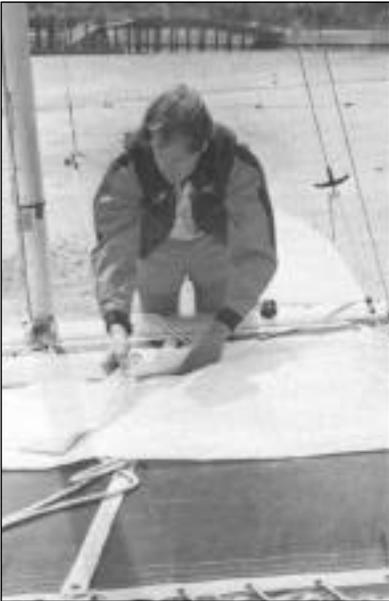
Roll tightly without any folds. If it is windy, put the jib under the hiking strap to keep it from blowing away while you lower the main.
