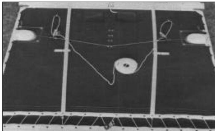
Hiking straps on trampoline are adjustable for personal comfort. People with long legs use the inboard look. Tie off onto a grommet at rear of tramp.
