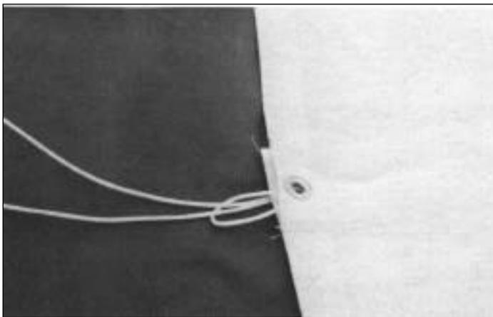
Fold batten string in half and loop through batten grommet on leech of sail.
