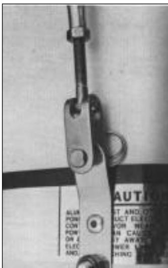
The turnbuckle on the diamond wire is attached to the lower fitting on the mast. The two separate turnbuckle studs should be started into the turnbuckle at the same time.
