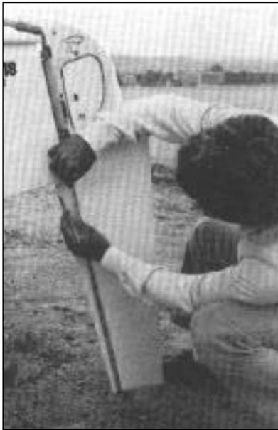
Lock both rudders down. Measure 20" up the leading edge of rudder and mark this measurement. Do the same on the trailing edge.
