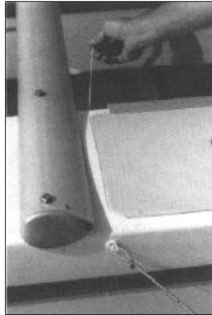
The trapezes are continuous from one hull to the other.
