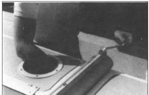
Align holes in front beam with the holes in the hull. Carefully thread all 4 of the 3/8" hex head bolts, with grease on threads, through the beam and into the hull until they are about 1/8" from being completely tight. CAUTION!!!
